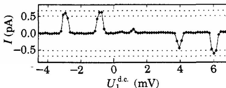
Fig.4. Dependence of the flowing current on the constant component of voltage at the first gate (H. Pothier et al., 1992)
