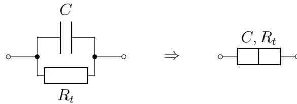
Fig. 1. Schematic diagram of a tunnel junction (left) and its representation in electrical circuit diagrams (right). The nonlinear element corresponds to a constant resistance  $R_t$  when tunneling is energetically favourable and to an open circuit (infinite resistance) when tunneling is impossible.
