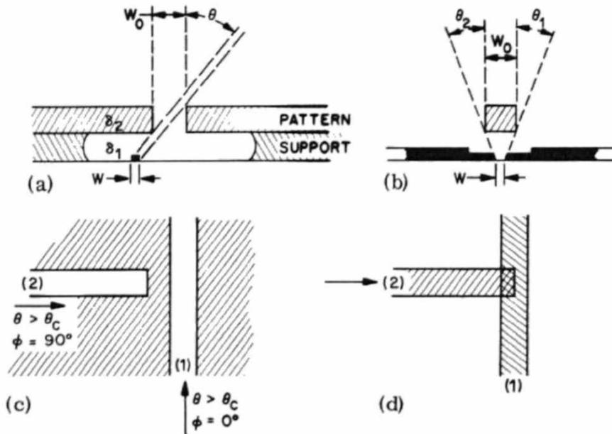
Fig. 1. Shadow deposition. G. J. Dolan, 1977.
