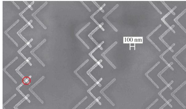
Figure 1. There are several tunnel junctions connected in series. One junction is circled in red. The figure shows three chains of tunnel junctions. The «check marks» that are not connected to each other are a side effect of shadow deposition technology. The picture was taken using scanning electron microscopy. M. Meschke et al., 2015
