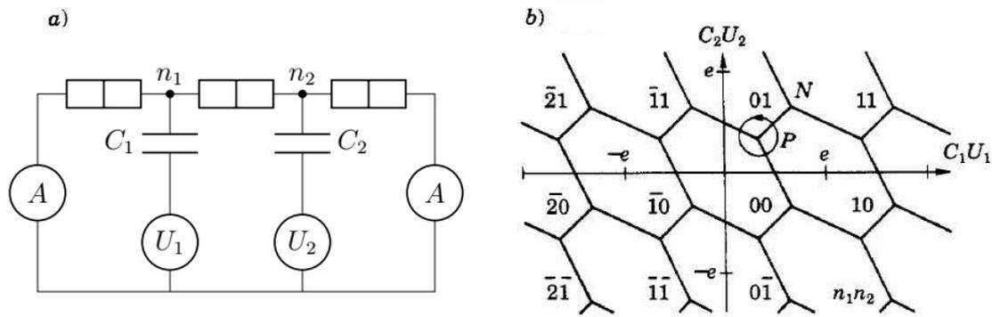
Fig. 3. Single-electron pump and its state diagram
